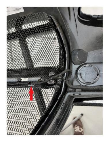
7. Once the grills are fully installed in the bumper and the PDC sensors have been reinstalled you will need to remove the outer layer of the two-piece bumper foam located on the aluminum crash structure on the front of the car.
